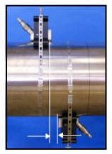
Figure 3-27: Distance Between Transducer Faces
